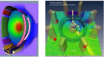
Neutron flux distribution and influence of the mascot robot inside the JET tokamak.
