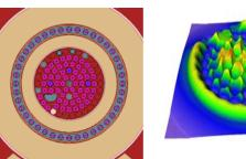
Computer model of the TRIGA reactor and sample thermal flux calculation.
