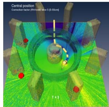
Neutron flux distribution and influence of the mascot robot inside the JET tokamak.
